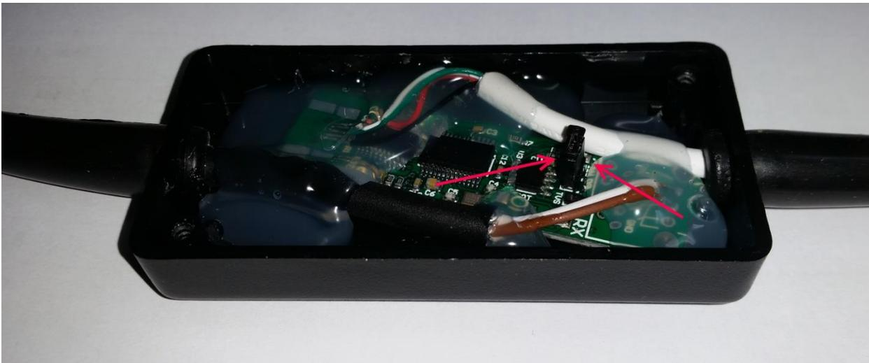
Please note: all GCU interfaces come with jumpers installed so if you're connecting to the existing CAN BUS, you need to remove the jumper.
