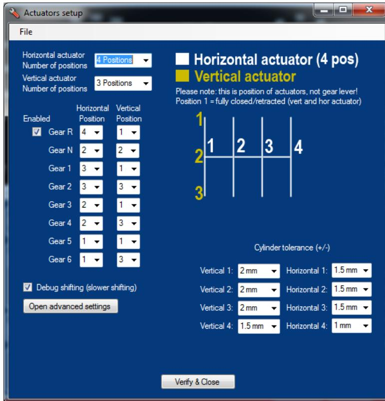
For each gear you need to set the position of each actuator.
