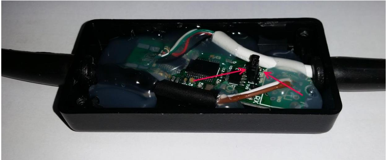
Please note: all GCU interfaces come with jumpers installed so if you're connecting to the existing CAN BUS, you need to remove the jumper.
