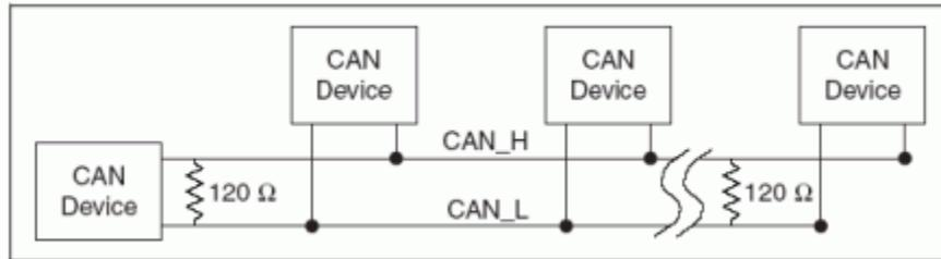
If you're connecting to a car that already has a CAN BUS, nothing is really needed, because your CAN BUS is already properly terminated. You just need to connect the CAN+ and CAN- to existing line and that's it.
