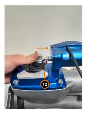
Pull the gear lever all the way that gearbox will shift gears. Measure the stroke. You need add space washers in the gear actuator that the gear actuator will stop before hitting the gearbox. (see GA-02, GA-03 manuals)
